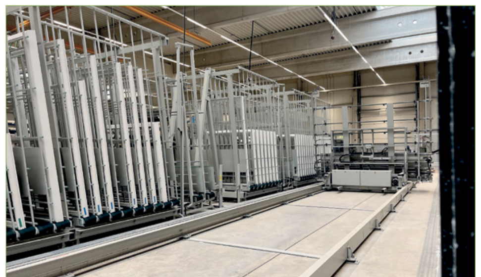
The elements are stacked automatically, thus making the best possible use of Urban's expertise.
