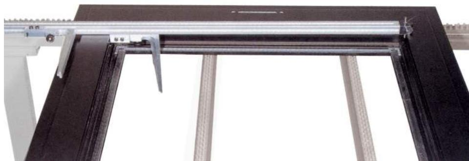
**Figure 2: Manual scanning with a length stop system** to ensure precise transfer of measurements for the cutting of the glazing beads with measuring bench that displays four movable measuring fingers, the four measurements for the glazing beads are scanned at the same time as length stops for the cutting (optional).
