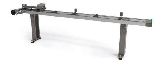
Roller is a loading roller conveyor with horizontal and vertical rollers for safe support of the profile. Extruded aluminum structure and adjustable feet. The support surface has a width of 220 mm, with four versions of length 3, 4, 5, 6 meters.
